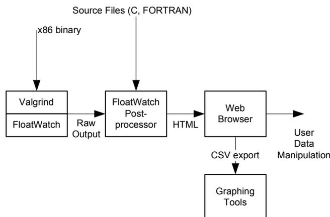
Figure 2: Block Diagram of the FloatWatch Tool Chain.
